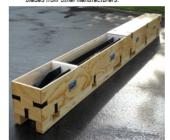
The top half of the dunnage secures the rotor blades in position. The long box top opens in two halves. The pallet runners are bevelled to enable dragging on uneven surfaces.
