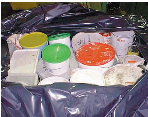
Paint is collected in a Clip-Lok container with an inner liner. UN approval obtained for 243 kg
