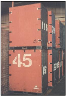
Custom designed to take different size detergent packages. The front panel has fixed clips. The boxes have made well in excess of 50 trips and are user friendly on high-speed packaging lines.
