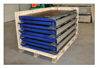
No space is wasted in this custom designed box. Special integrated dunnage keeps the flood barriers in place to prevent damage under transport.
