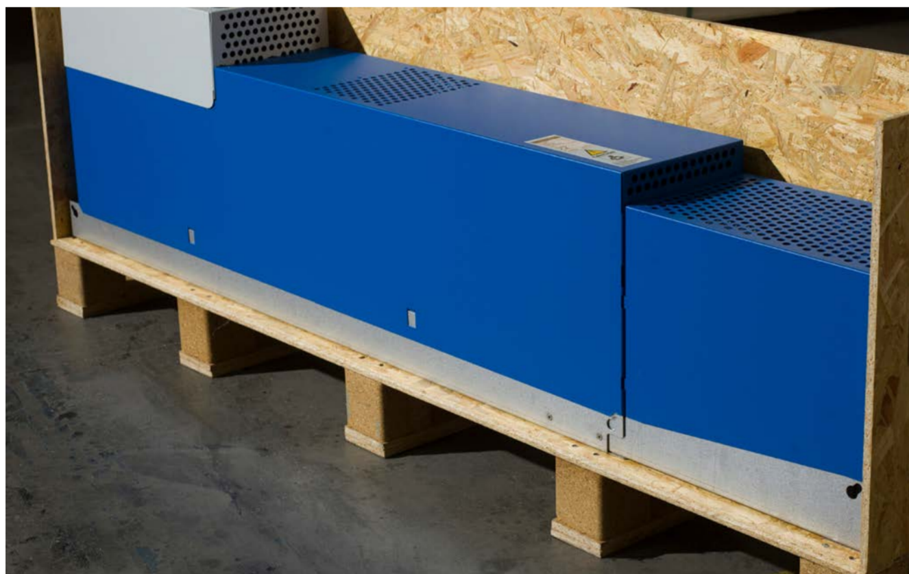
The Clip-Lok Expendable box loaded with two power quality units and bolted at the pallet base.
