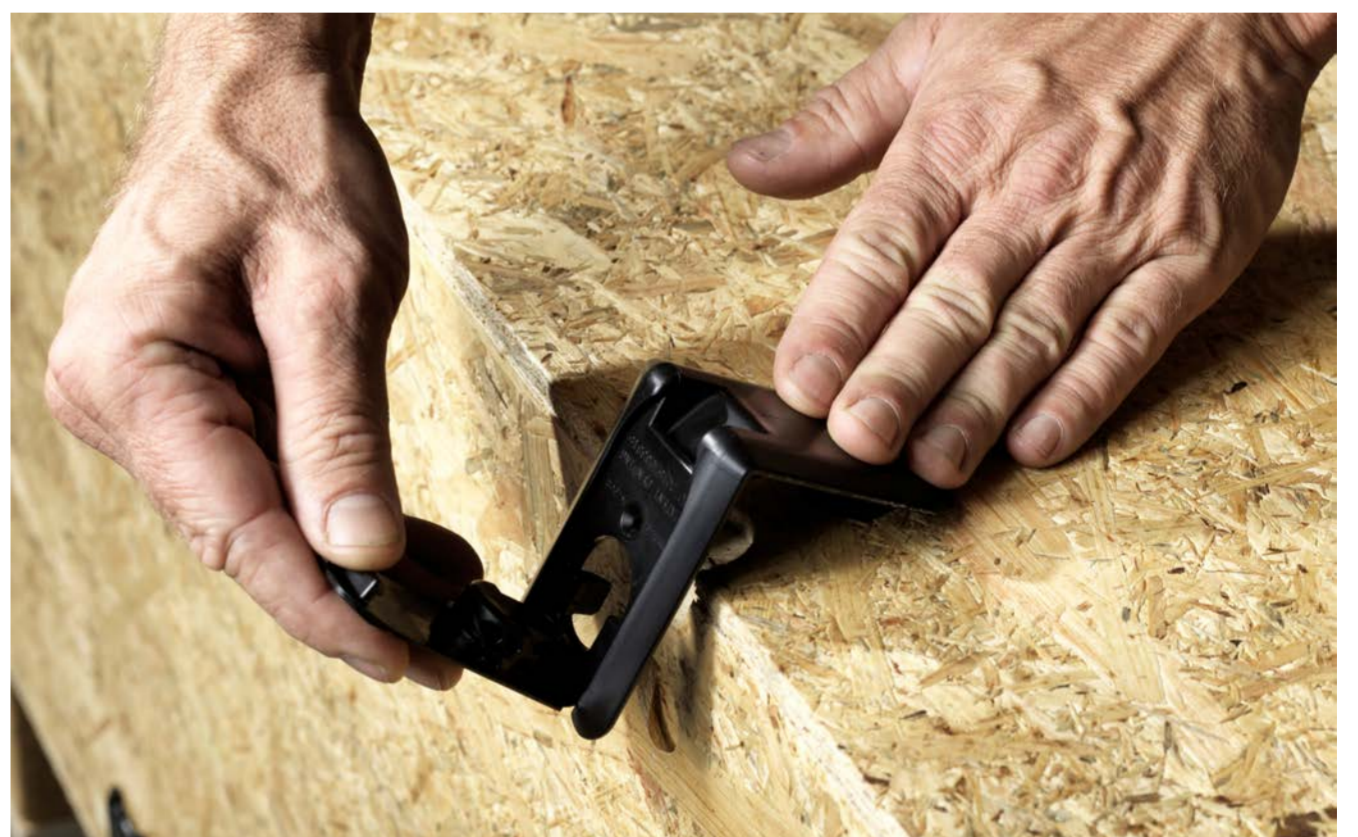
Clip-Lok QIK Plastic clip requires no tools while assembling or disassembling the box, ensuring a tool free environment.
