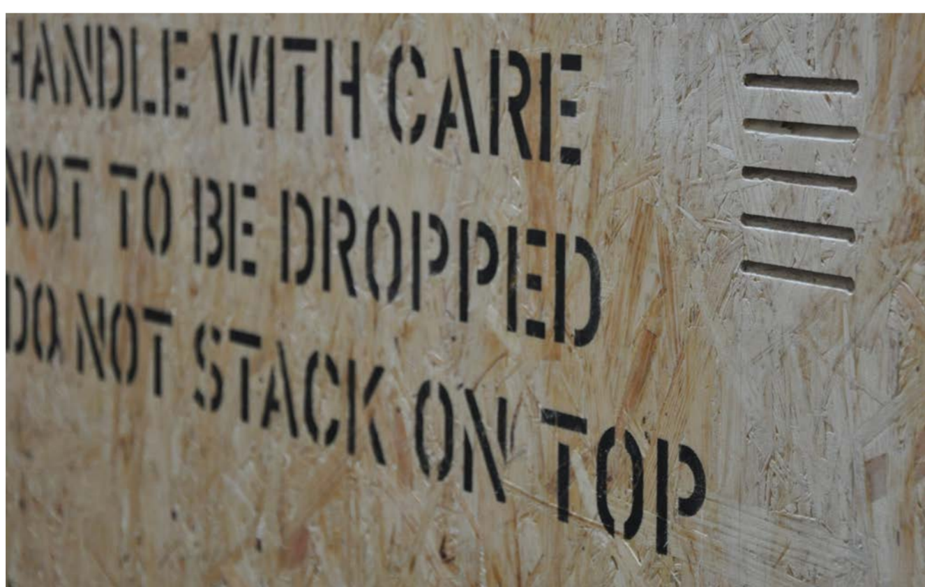
Strategically placed air vent to control heat inside the box during transport.
