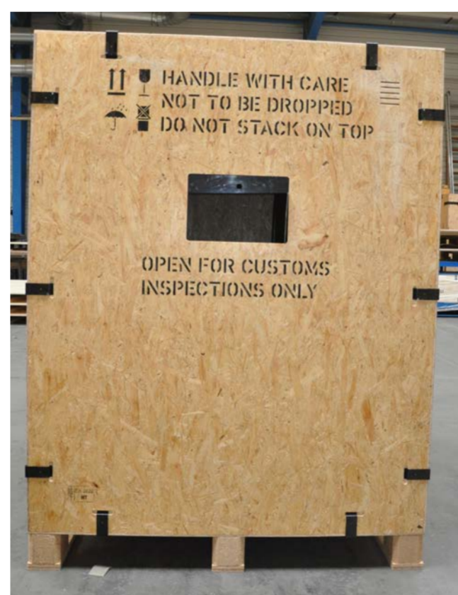
Inspection hole on the side for custom checks for easy custom clearances. The Clip-Lok QIK Plastic clips showcasing ease of use and creating a tool free environment.
