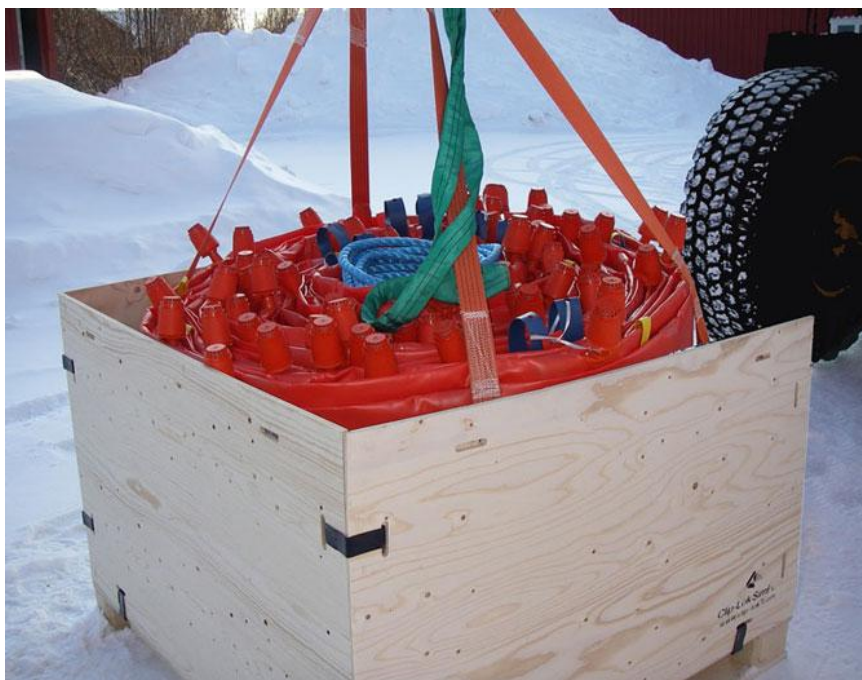
The oil boom can easily be handled by crane without removing all panels
