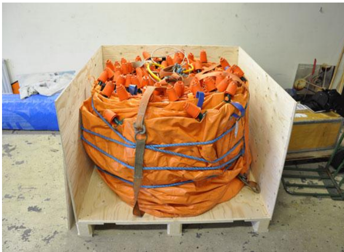
The size of the Clip-Lok box matches the volume of the oil boom. The oil boom can be handled from the side and top
