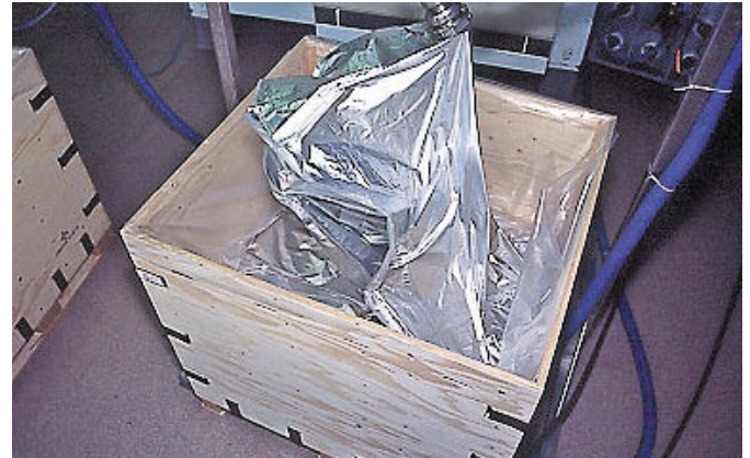
Above: The barrier bag and the liner ready for filling
