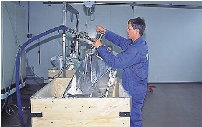
Above: Fitting the connector rod to the bag
