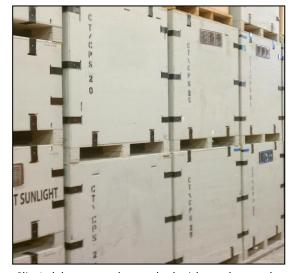
Clip-Lok boxes can be stacked without the need for racking.
