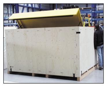
*Left:* The box being built around the unit, the lid of which is then closed
