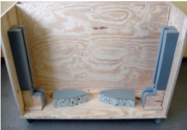
The foam dunnage on which the TV rests is fixed to the base and ends. It allows the side to be removed while the TV is still safely secured in the foam.
