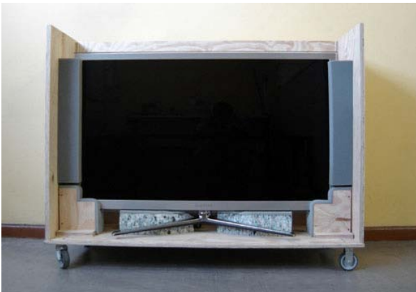
TV loaded in the box. The box can be opened from the top or side. Wheels attached for easy moving
