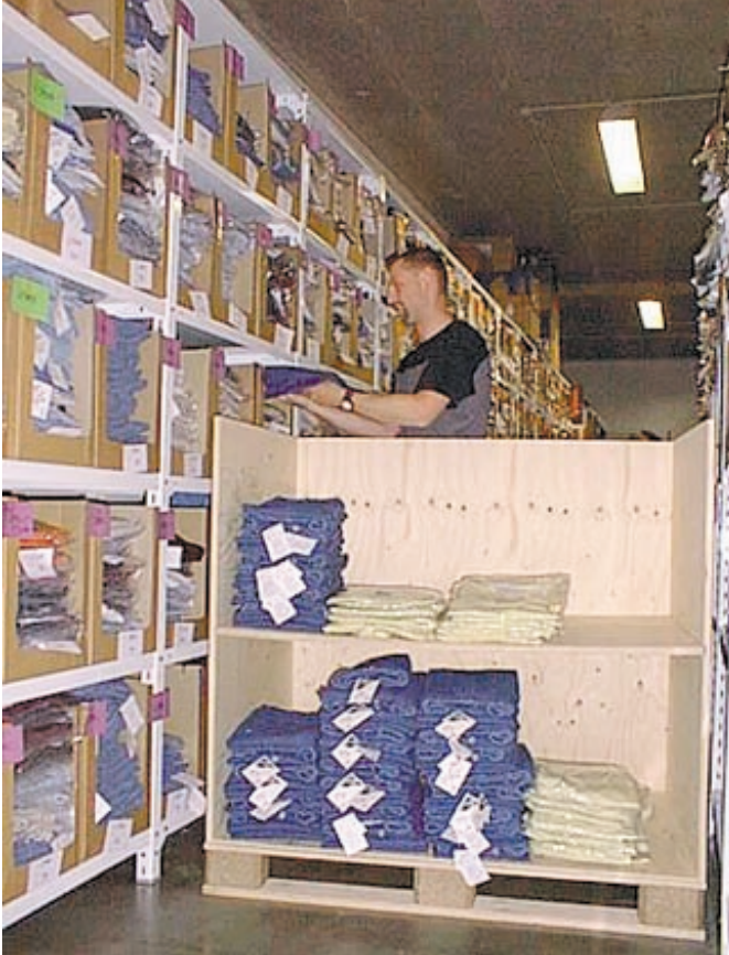
Above: Overalls for Rie Design Aps: the shelf prevents creasing of clothing on the bottom and removable panels facilitate easy packing.
