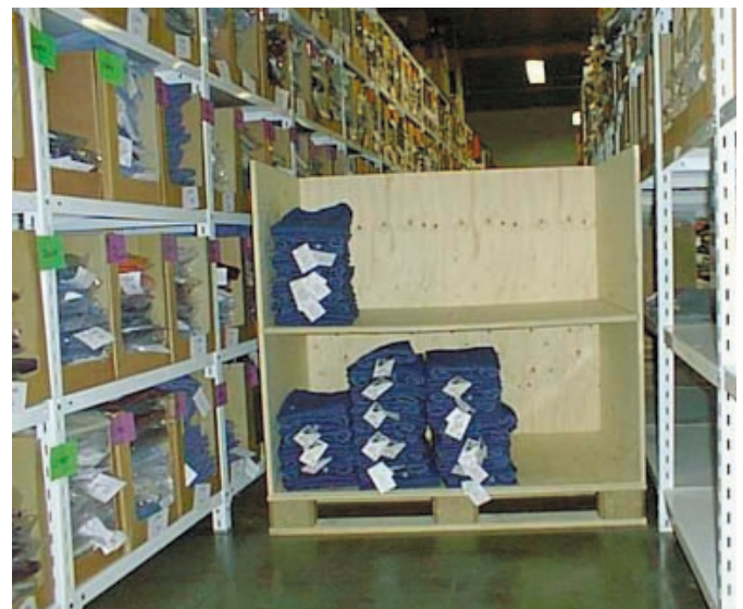
Below: Clothing for Fristads Ab: boxes with half-panels which can be removed easily to allow for packing from top and front.
