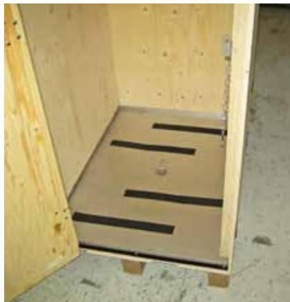
The hygienic platform is placed in the bottom of the box, ensuring water is lead from the cabin
