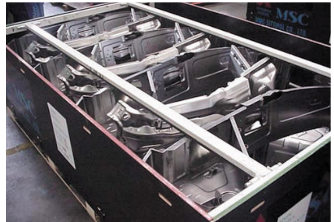
Above: Tailor made dunnage holds parts secure
