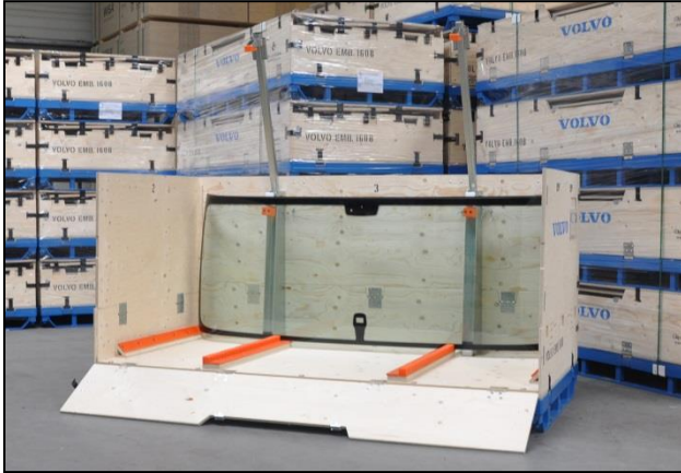
The integrated steel and polyurethane dunnage folds into the box when flat-packing. The spring steel clips are hinged on the panels for easy handling.
