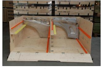
Both the right and the left door part can be packed in the same box. Protective PUR dunnage and felt are especially important once the parts are painted.
