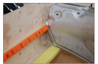
The metal door parts rest on a protective felt-lined shelf. This is especially important for preventing scratches or friction marks once the parts are painted.
