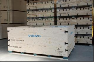
When the lid is placed and secured, the box will be ready for shipment. Behind the loaded box are stacked flatpacked boxes. The integrated pallet base allows 4-way handling.
