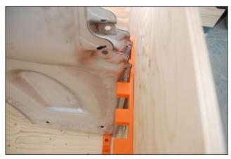
Robust polyurethane dunnage cradles each door part to prevent damage while maximizing packing density.
