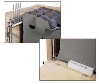
Custom-designed dunnage carries the panels in precise position and secures them under transport.
