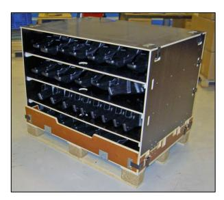
This Clip-Lok 2P box has specially designed shelving to hold layers of petrol tank filters. The easy access and the removable shelving make this box ideal for Just-In-Time and in-sequence delivery and Lean manufacturing.
