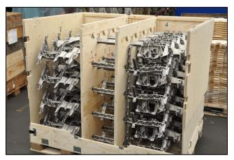
The dunnage is built-up in sections providing easy access to the parts. When in place, the dunnage firmly secures each part in position within the box. This ensures maximum packing density while preventing damage during shipping.
