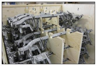
The box is shipped directly to the assembly line where the workers have direct ergonomic access to the parts.
