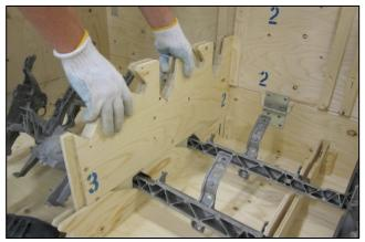
The rack can be build up/taken down as the items are loaded/unloaded. Expert craftsmanship and finishing work ensure that the box will hold up under many return transports.
