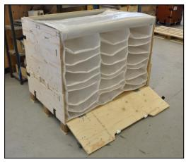
Once on the production line, the box is easily opened giving direct access to the instrument clusters. Without any further steps such as unwrapping parts, the operator can continue the assembly process maintaining an optimized flow.
