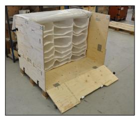
Here the front rack has been removed giving access to the next rack. The waste-free Soft Rack dunnage solution replaces traditional plastic bubble wrapping which has to be removed and discarded upon arrival.
