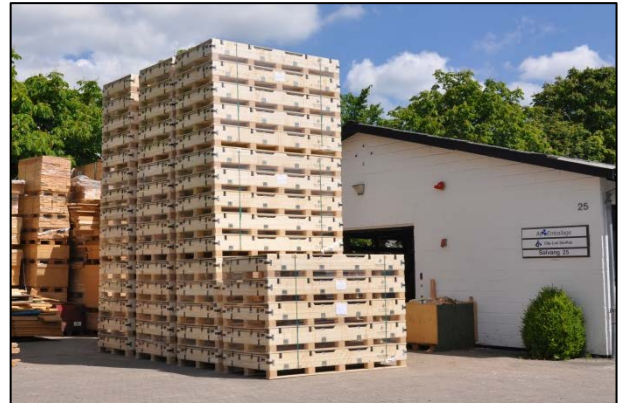
The custom designed plywood dunnage is 35% stronger than the cardboard alternative, providing better support and security to the Busbars during shipping and thus saving costs.
