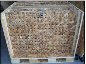
In this photo, all of the dunnage is in place with just one camshaft loaded to show the packing density of this custom designed packaging.
