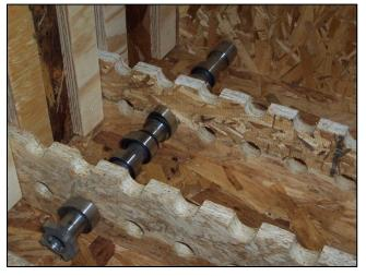
The camshaft is held securely in place between the grooved supports. The supports are slid into place as each layer of camshafts is built up. This system allows fast and easy packing and unpacking of the parts.
