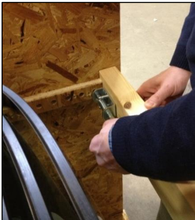
An adjustable spring-loaded bolt lock secures the windshields regardless of the number of windshields being transported.
