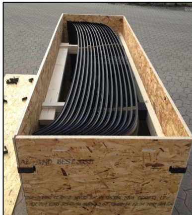
A full load of 15 windshields are held securely in place. The unique dunnage and closed box design will protect the glass and primer from damage under transport.
