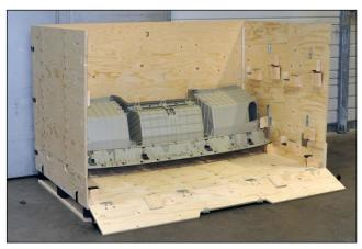
Once on the production line, the box is easily opened giving direct access to the parts. Without any further steps such as unwrapping parts, the operator can continue the assembly process maintaining an optimized flow.
