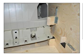
Specially designed protective dunnage holds the shelves securely in place and allows easy access on the production line.
