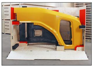
The final panel is secured in place and the box is ready for closing. The access ramp folds up and the top and side of the box can be easily clipped into place.
