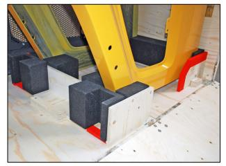
Plywood, foam and felt dunnage keep the parts separated and secured. The sensitive lacquered parts are fully protected from damage.
