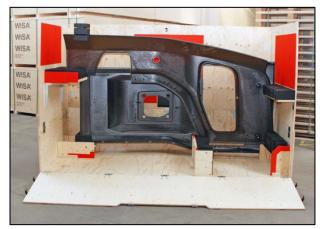
The first two panels are loaded into the box. Custom designed dunnage ensures that the panels cannot come in contact with each other.
