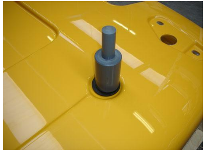
The roofs are separated with spacers in each corner. The spacers are easy to place between each roof
