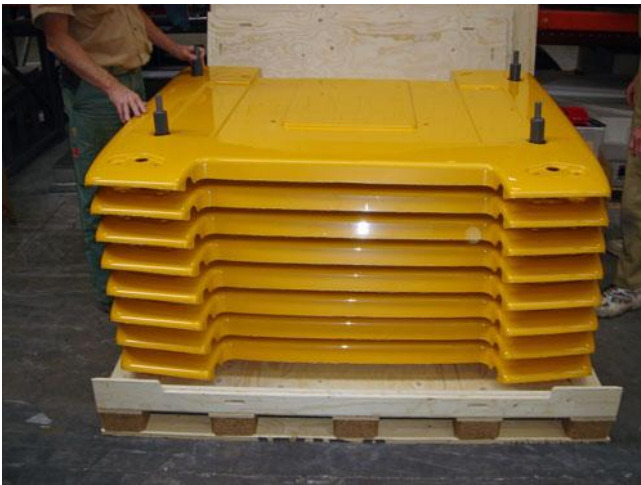
The spacers allow several roofs to be placed on top of each other with out the risk of damage during transport
