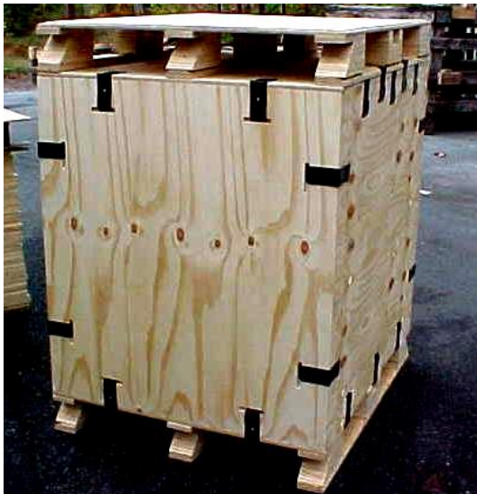
The chamfered blocks are used for chain handling
