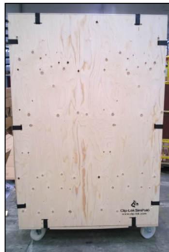
The box is packed and ready for shipping. Heavy-duty plywood and spring steel clips ensure safe transport of the cots.
