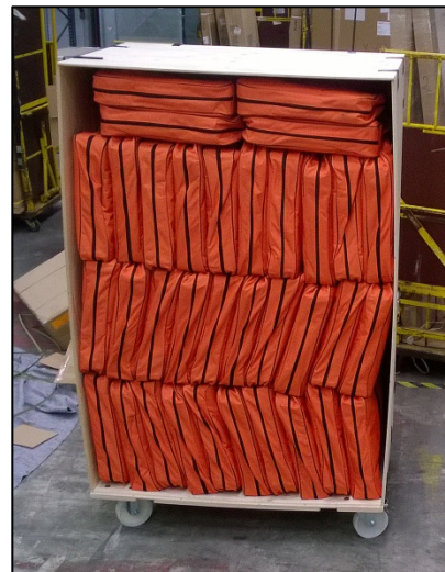
The Clip-Lok wheeled box holds 34 collapsed cots. Here, the front panel of the box is removed for easy loading access.
