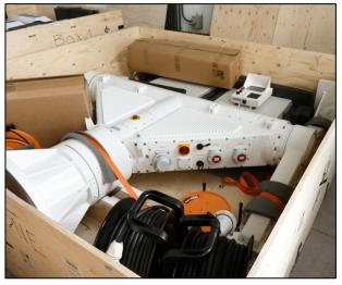
A heavy and bulky mainframe is held in place with special dunnage and straps. The space around the main frame is used for various accessories.
