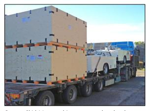
Orange Skid-Mate cushions mounted under the boxes absorb shock and vibration to further protect the electronics under transport.
