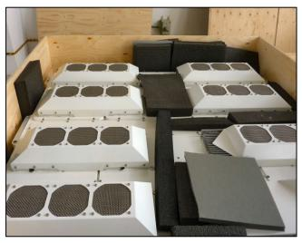
The radar discs are packed separately. The clipped box has smooth surfaces and no nails which could damage the discs.
