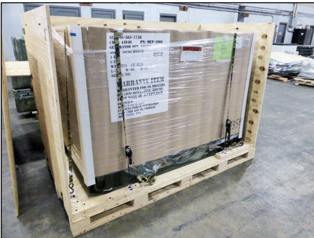
Heavy duty plywood ensures safe transport of the generators, which weigh between 1,500 and 5,000 lbs. (680 to 2,268 kg) each.
