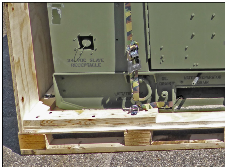
Heavy duty plywood ensures safe transport of the generators, which weigh between 1,500 and 5,000 lbs. (680 to 2,268 kg) each.
