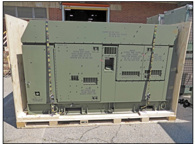
Once the front and top panels are clipped into place, the box will be ready for outdoor storage in all types of weather.
