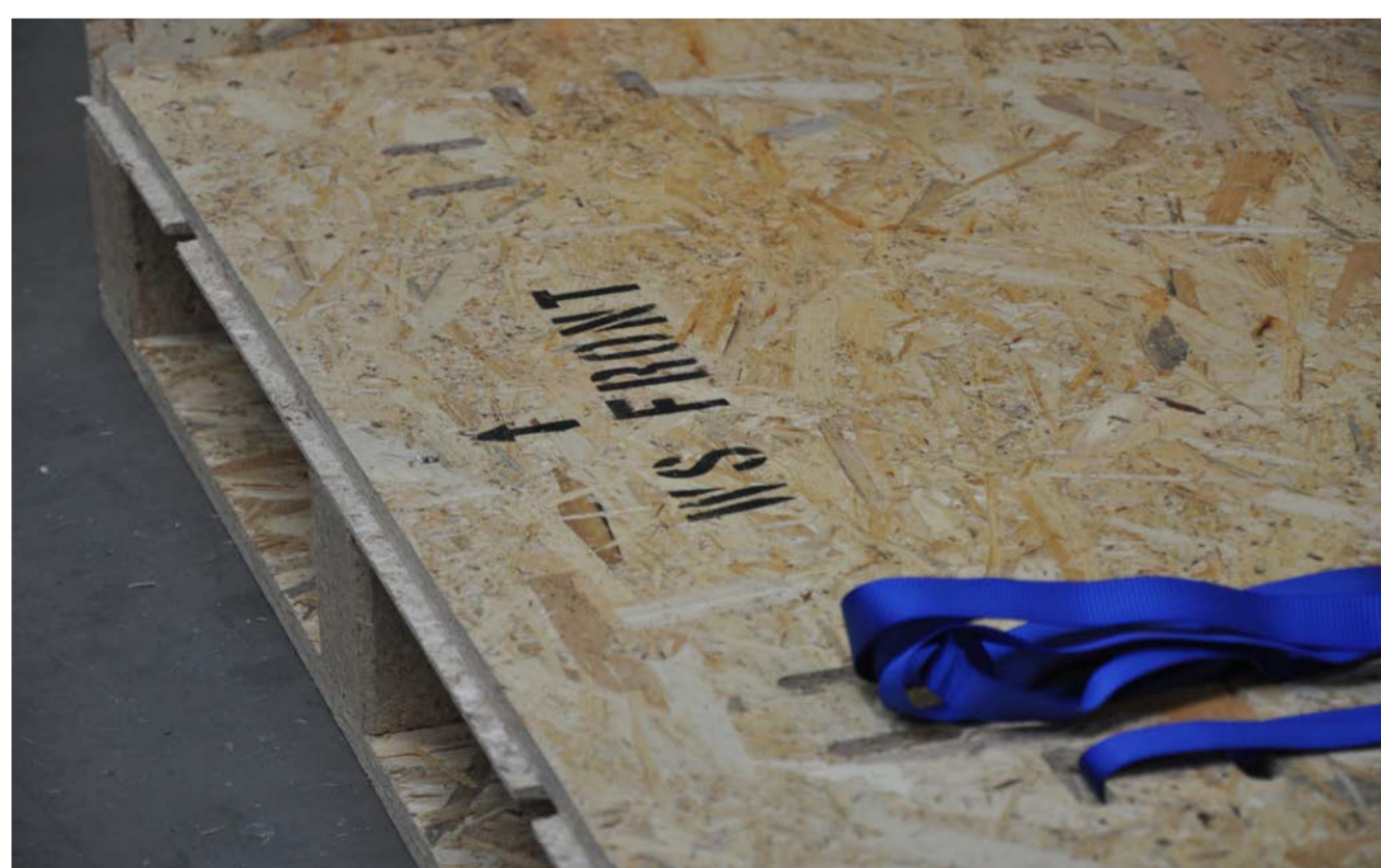
Strap connectors are imbedded in the base of the box to secure additional equipments.
