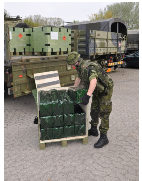
The box can easily be loaded or emptied with two open sides
