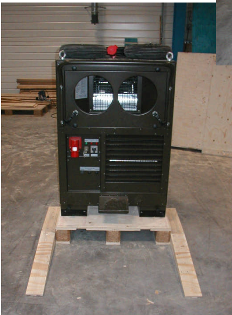
When the A/C is loaded the wheels are detached and placed on the top
