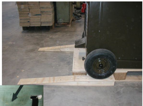
Wheeled on to the pallet base by the use of attachable ramps
