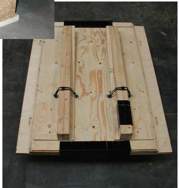
Flat packed box with ramps tightened to the side of the box. Spare clips on runners
