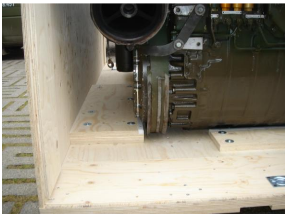
Mounting blocks and straps for stable and safe transport
