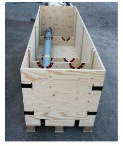
The felt-protected plywood dunnage slides easily into place as layers of missiles are added.
