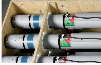
Plywood and felt dunnage keep the missiles separated and securely loaded. They are fully protected against damage, including the painted and sensitive surfaces.
