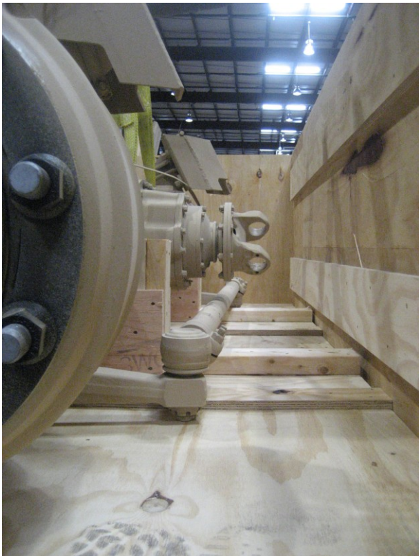
The design of the Clip-Lok box allows easy access when loading the axle with forklift
