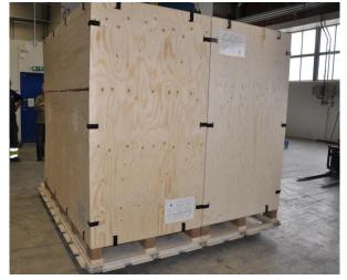
The box panels can be easily removed as needed. This allows loading from the top or side, or on an empty pallet if all sides are removed.
