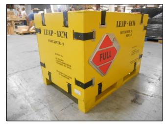
The box is painted with epoxy paint and printed with a logo and information. A reversible sign is used to indicate whether the box is full or empty. Hinged clip retainers keep the clips fastened to the box panels.
