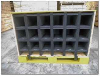
There are 18 numbered compartments on each side of the box, so 36 nozzles can be transported in each box. The box can be opened from either side.
