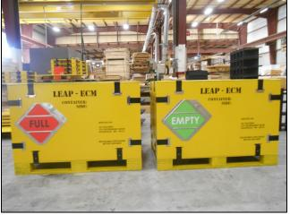
Heavy-duty plywood and spring steel clips ensure safe transport of the nozzles. Worn or damaged box panels are replaceable, extending the life and economy of the box. The integrated pallet base allows 4-way handling.
