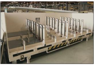
Plywood and foam dunnage keep the ribs separated and securely loaded. Even the painted and sensitive surfaces are fully protected from damage.
