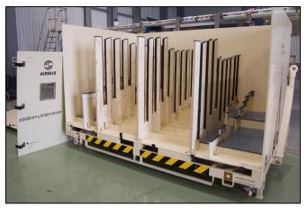
Each of the boxes in the series holds a set of eight different ribs. The custom designed boxes provide optimum packing density.
