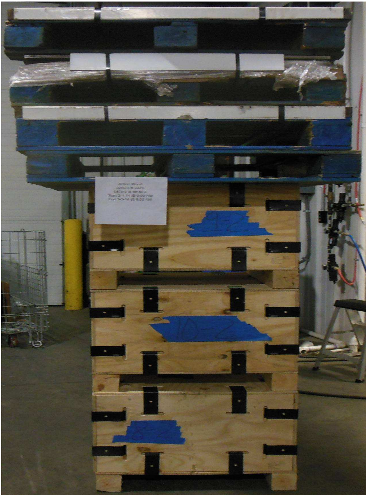
Stack load testing
