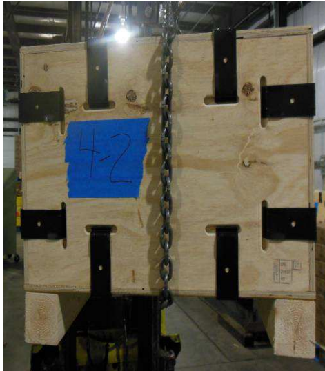
Bottom Drop (Face 3) Test sample 4
