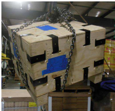
Bottom MFG Joint Corner Drop (Corner 5-3-2) Test sample 8
