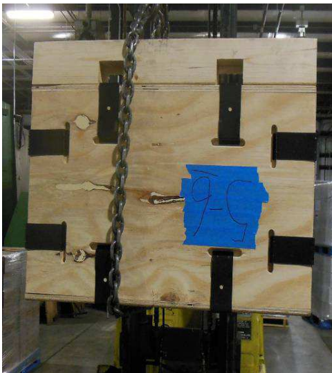
Top Drop (Face 1) Test sample 5
