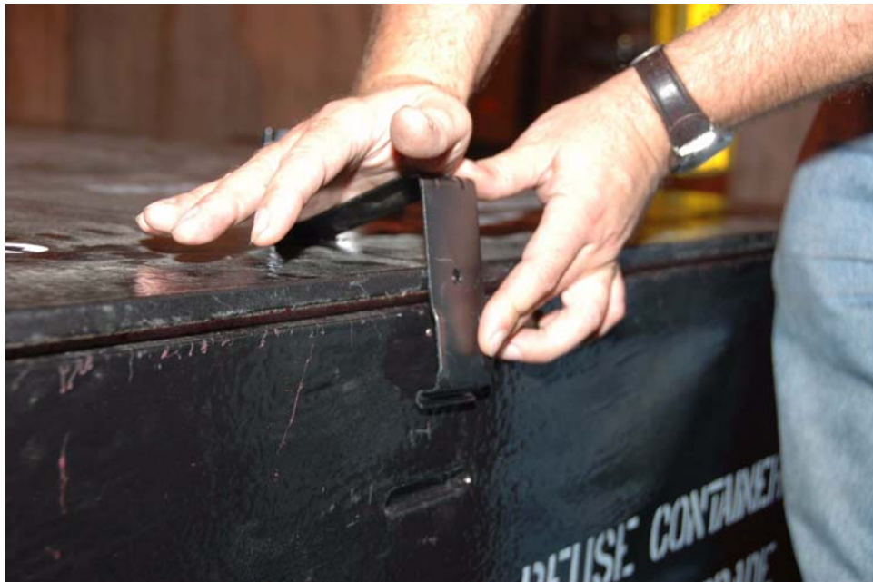
Figure 3. Steel Clip Securing the Lid to the Base
