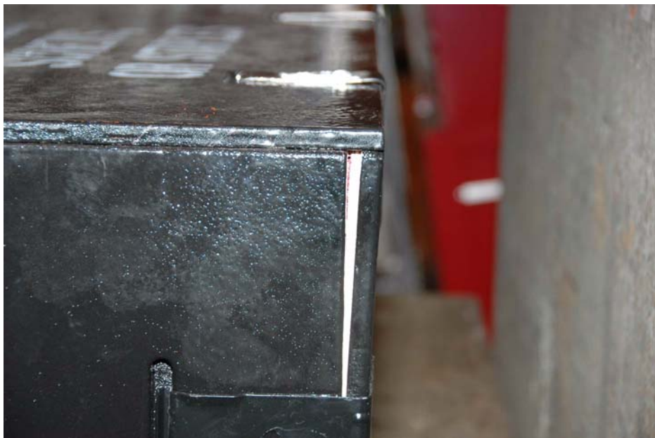
Figure 10. Misalignment of Panels Near Base After Incline Impact Test
