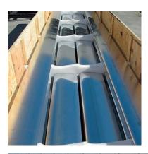
This 5 meter long box can hold 16 blades held securely in place by sturdy polyethylene foam dividers.
