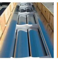
This 5 meter long box can hold 16 blades held securely in place by sturdy polyethylene foam dividers.
