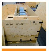
The heavy IGBT stacks are cradled in shock absorbing high density polyethylene foam and robust plywood panels.
