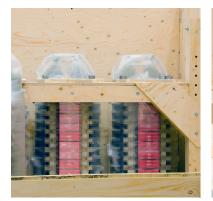
The adjustable top crossbar can support chopper valves of various heights. All of the dunnage fits in the bottom of the box. Product images are blurred to conceal design details.
