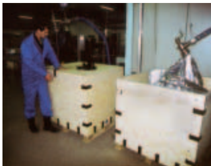
■ Fish oil is pumped into a 1,000 litre (300 gal) disposable plastic bag for discharge on delivery through the fast-flow outlet valve at the bottom.
