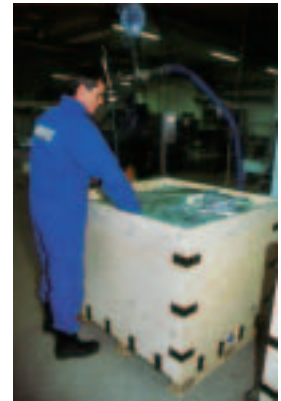
■ Liquid box capacity of 1,000 litres (300 gal) replaces 4 disposable drums.
