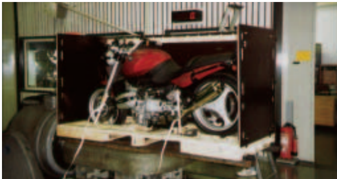
■ Vibration tests on box for motorbikes.
