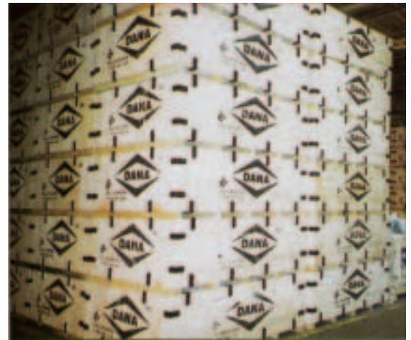
■ Boxes weighing 3,200 kg (7,200 lbs) stacked six high without racking.
